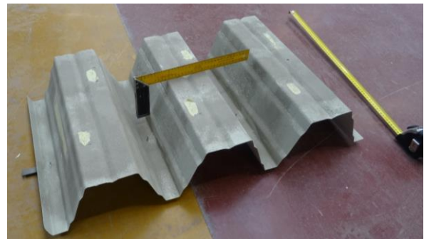
Fig. 14 Trapezoidal sheeting covered by concrete dust
