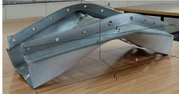
Fig. 5 Permanent deformation measurements (Ref. 13)
