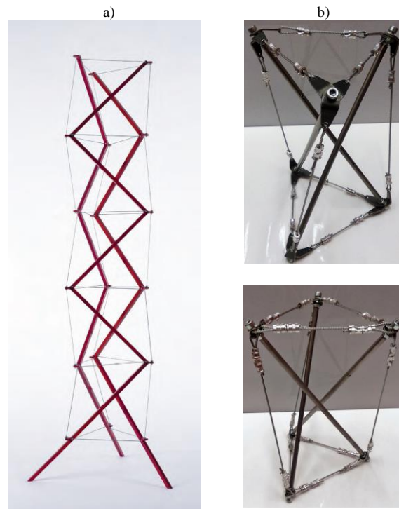
Fig. 1 a) the Snelson's sculpture (Ref. 1), b) the left-handed simplex (top) and the right-handed simplex (bottom)
