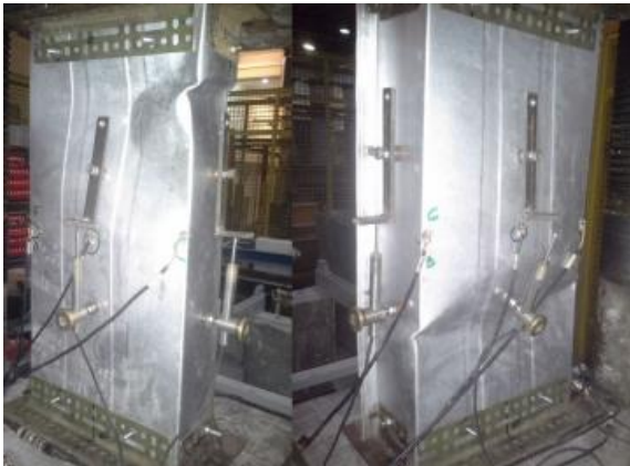
Fig. 17 Straight panel: experimental deformation shapes
