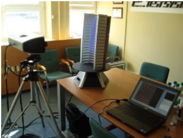
Fig. 11 Set-up for 3D scanning
