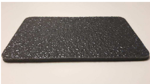
Fig.3 Photo of a typical polyurea sample with non-slip surface [2]
