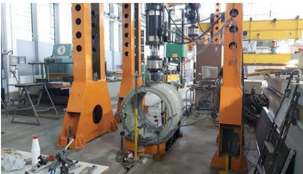
Fig. 6 Frame used in testing concrete rings
