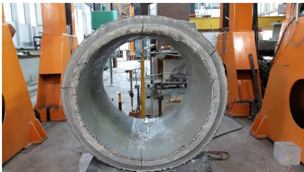
Fig. 9 Concrete ring with polyurea coating on external and internal surface after destruction and unloading
