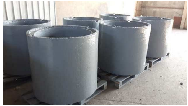
Fig. 2 Tested concrete rings covered by polyurea coating system
