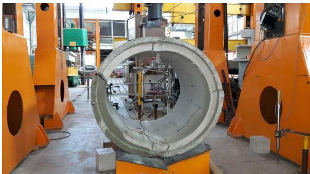
Fig. 8 Concrete ring with polyurea coating on external surface after destruction and unloading
