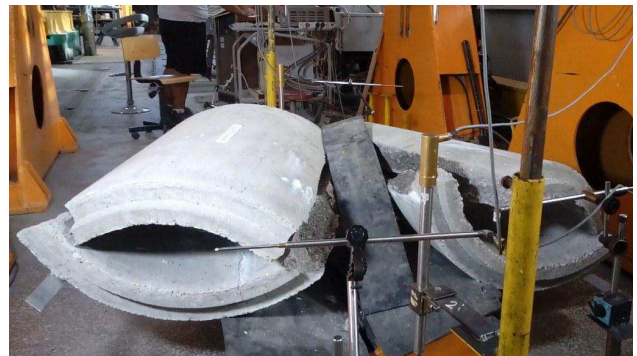
Fig. 7 Concrete ring without any additional coatings after destruction
