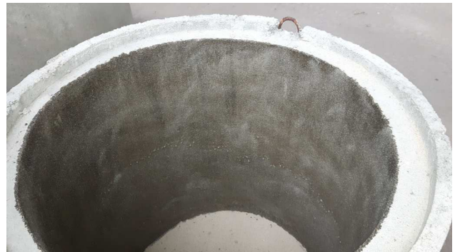
Fig. 3 Sample of concrete ring covered by special primer suitable for concrete surface in combination with dried quartz sand
